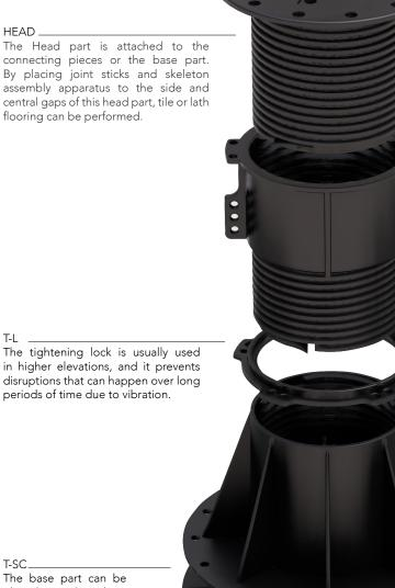
After 181 mm, products are heightened by connecting pieces. More than one piece per module can be used. Electricity wiring and waterwork can be tied to the side and upper parts of these products. This allows for easy access and technical efficacy by holding the installations higher than the ground.
